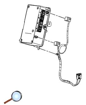
3. Disconnect the VCIM electrical connectors as necessary.
